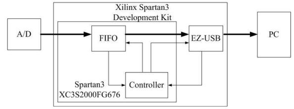
Fig. 7. Function block diagram for USB communication
