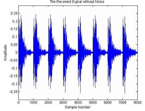
Fig. 4. The UWB channel and the received signal
