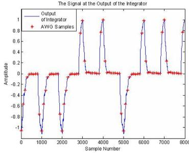
Fig. 6. The signal after the integrator
