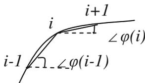
**Fig. 5** The sampling points on the output curve of the ADC
