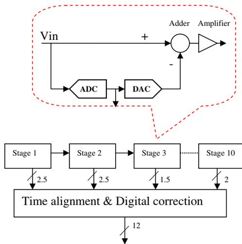
**Fig. 6** The basic structure of a 12-bit pipelined ADC
