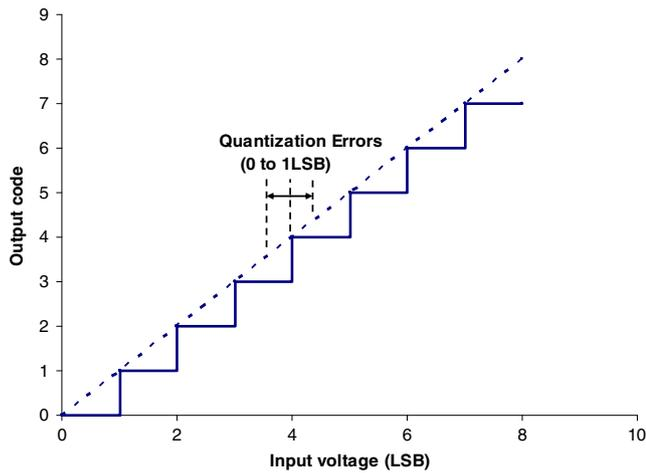
**Fig. 1** Ideal transfer function of a 3-bit ADC
