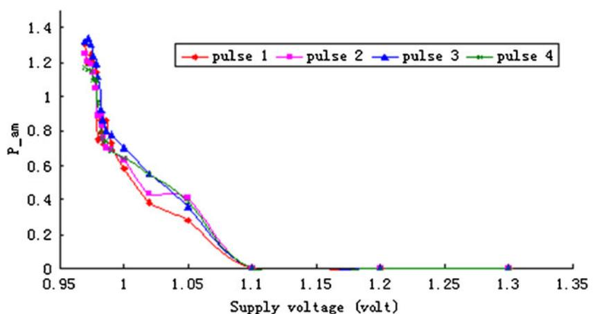
**Fig. 13** Measured  $P_{L\phi}$  of the 12-bit pipelined ADC vs. supply voltage
