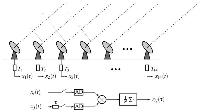
Figure 1: Schematic of the Westerbork radio telescope
