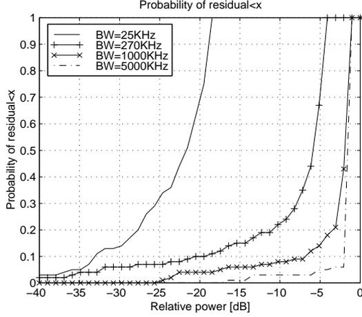
Figure 2: Probability distribution of relative residual power.  $BW = 25$  kHz, 270 kHz, 1 MHz, 5 MHz. FM chirp.
