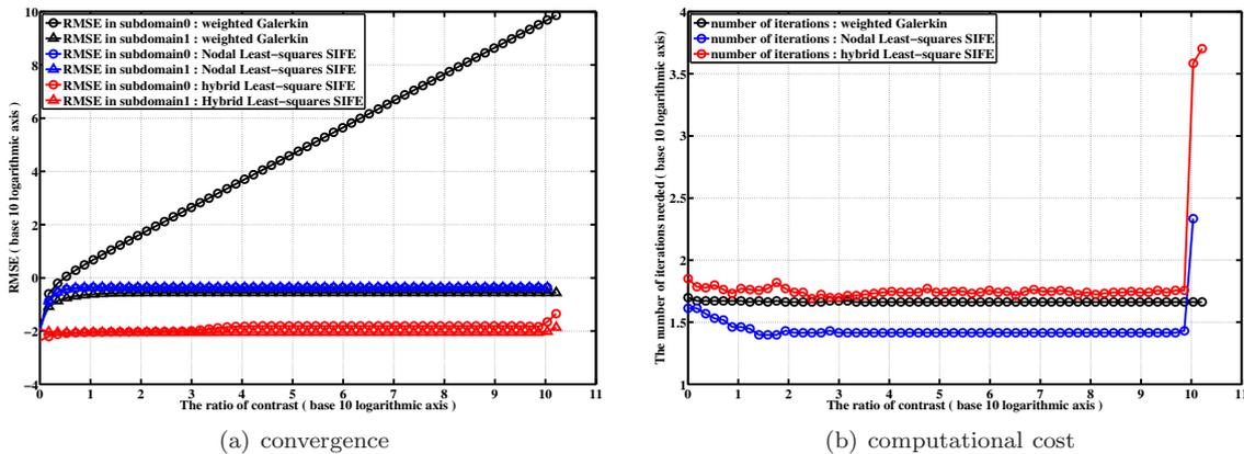
Figure 3: The relative root mean square error in  $\mathcal{D}_0$  and  $\mathcal{D}_1$  vs. the ratio of contrast (a). The number of iterations needed by iterative linear solvers versus the ratio of contrast; BICG-stable + nested dissection reordering + ICC(2). the accuracy of the iterative linear solver:  $1 \times 10^{-12}$ (b).
