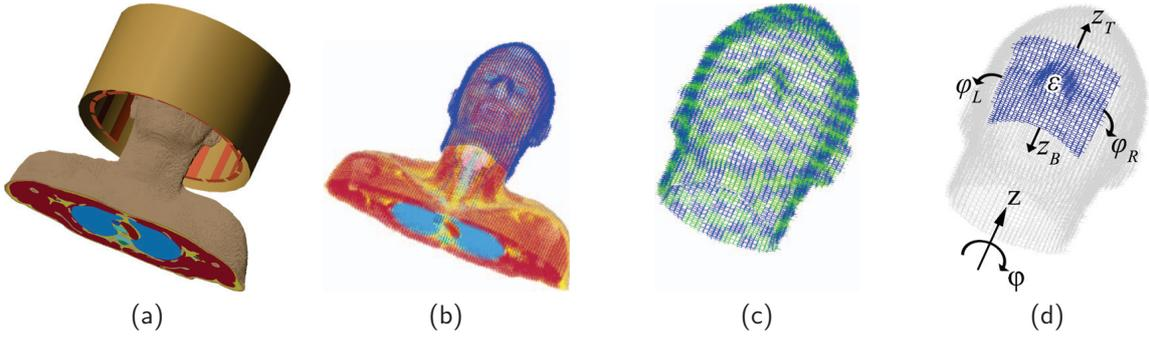
Figure 2: Head and shoulders of the male body model Duke, head coil, and shield used for enhanced imaging of the cerebellum (a). The pad design domain defined all around the head model (b). Pad design domain subdivided into subdomains (c). Illustration of the pad design parameters (d).
