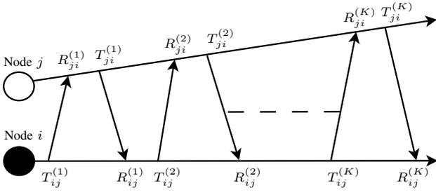
Fig. 1. This figure shows the classical two way communication between a node pair  $(i, j)$ . Node  $i$  is the reference with  $[\omega_i, \phi_i] = [1, 0]$  and also initiates the communication with node  $j$  whose clock skew ( $\omega_j$ ), clock offset ( $\phi_j$ ) and distance ( $d_{ij}$ ) from node  $i$  are unknown. There are  $K$  two way communications between the node pair during which  $2K$  time markers are recorded at the respective nodes.
