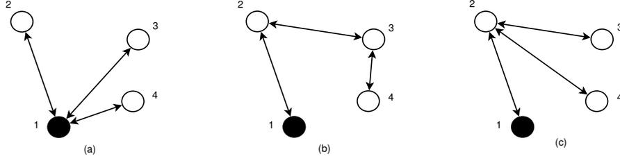
Fig. 3. An illustration of 3 networks with  $N = 4$  nodes each capable of two way communication. The node shaded in black is the clock reference. The 3 networks are illustrative examples where GLS algorithm can be applied for network wide clock synchronization, despite missing communication links.
