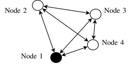
Fig. 2. An illustration of a network with  $N = 4$  nodes, each capable of two way communication. Node 1 (shaded in black) is the clock reference with  $[\omega_1, \phi_1] = [1, 0]$ . The clock skews and clock offsets of node 2, 3 and 4 are unknown and are to be estimated, in addition to all the pairwise distances.
