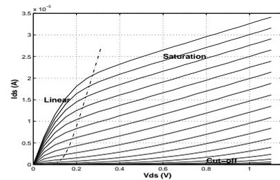
Fig. 2. The nonlinear properties of minimum-sized NMOS device
