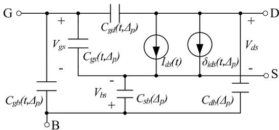
Fig. 1. The proposed SXmodel for gate modeling
