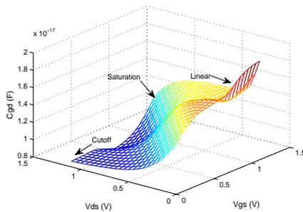
Fig. 3. Non-linearity properties of  $C_{gd}$  of a 45nm NMOS transistor
