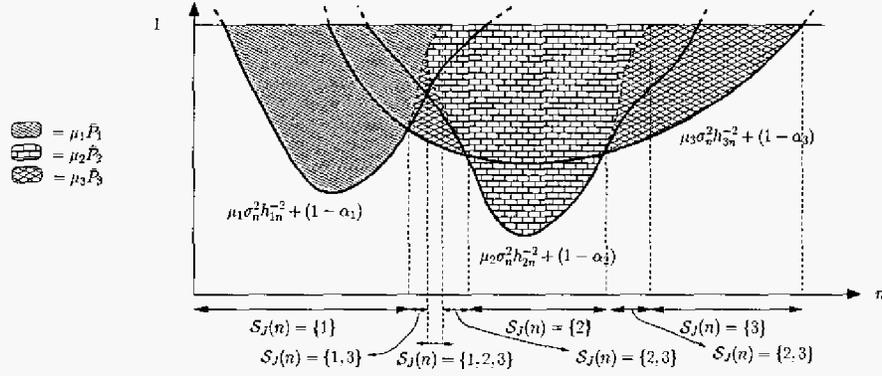
Fig. 1. Multiuser water-filling diagram
