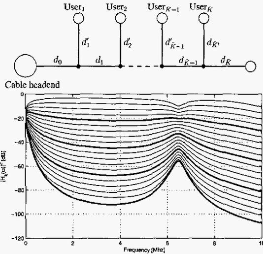
Fig. 3. Wireline multiaccess network and associated channel responses
