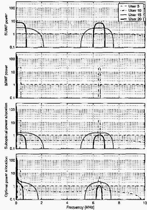
Fig. 4. Normalized power allocations
