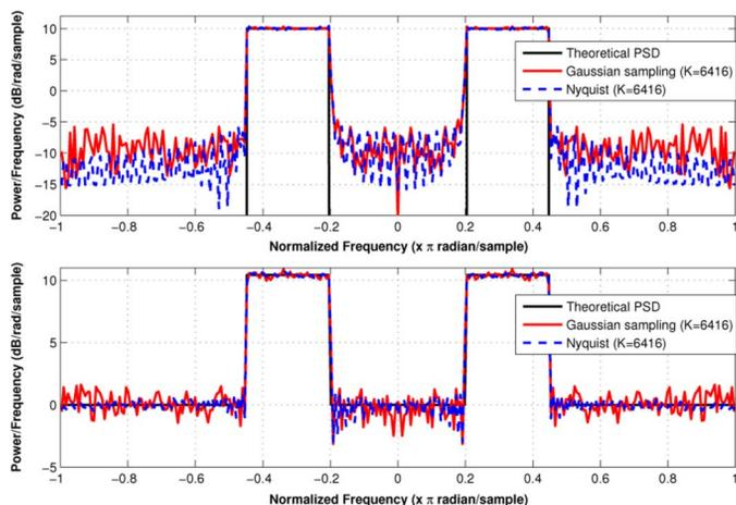
Fig. 3. Power spectrum estimated based on PSBS with  $M/N = 0.5$  is plotted together with the theoretical and Nyquist-rate based power spectrum; top: noise-free; bottom: noisy.
