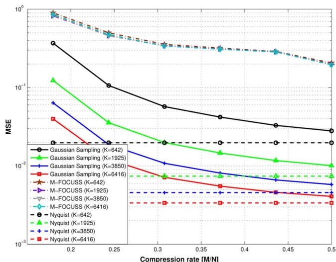
Fig. 2. MSE between the PSBS-based power spectrum and the theoretical one.
