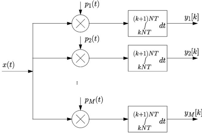
Fig. 1. Considered sampling device, consisting of  $M$  branches, where each branch modulates the signal with a real-valued periodic waveform followed by an integrate-and-dump process.
