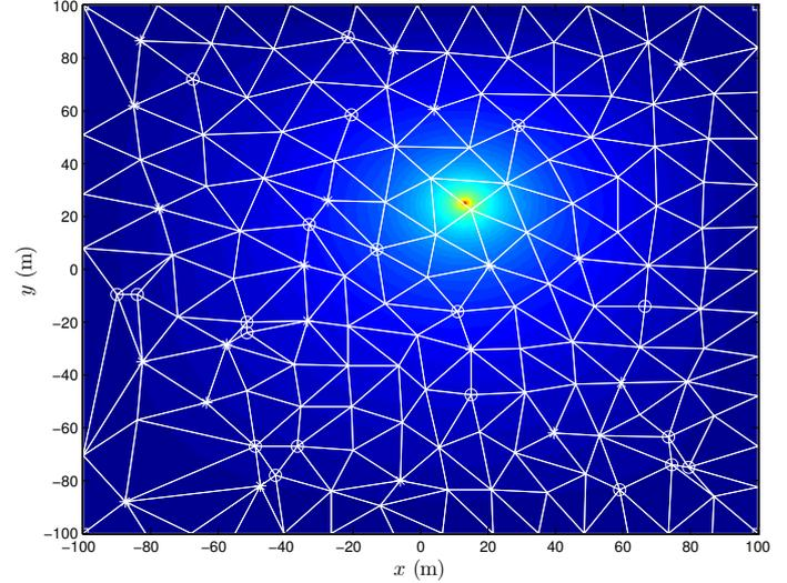
Fig. 1. Contour plot of the simulated field showing a FEM mesh generated for one realization of the random sensor node and POI deployment. A fixed subset of the FEM nodes consists of WSN sensor nodes (o), POIs (\*), and domain corners (□).
