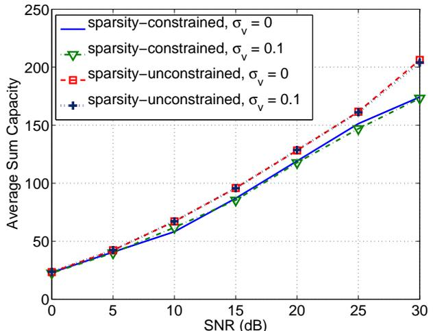
**Fig. 2.** Average sum capacity vs. SNR budget (decided by  $P_{q,\max}$ ) for both sparsity constrained and unconstrained DRA games, when sensing errors are zero ( $\sigma_v = 0$ ) or moderately large ( $\sigma_v = 0.1$ ).
