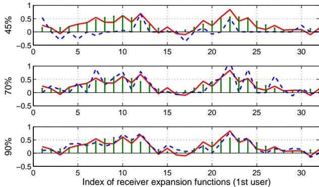
**Fig. 1.** Noise free interference profile (vertical lines), its noisy realization (dashed line) and the estimated interference (solid line) versus the function index, for user  $q = 1$ .
