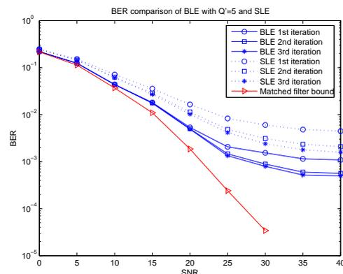
Figure 4: BER comparison of low-complexity block turbo equalizer and SLE
