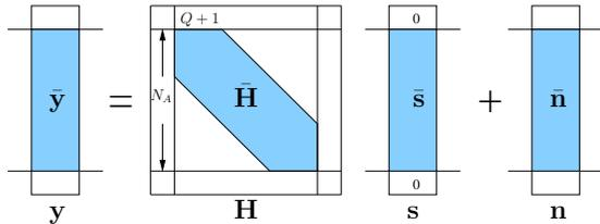
Figure 1: System input-output relation after removing the guard intervals
