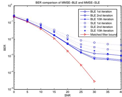
Figure 3: BER comparison between BLE and SLE
