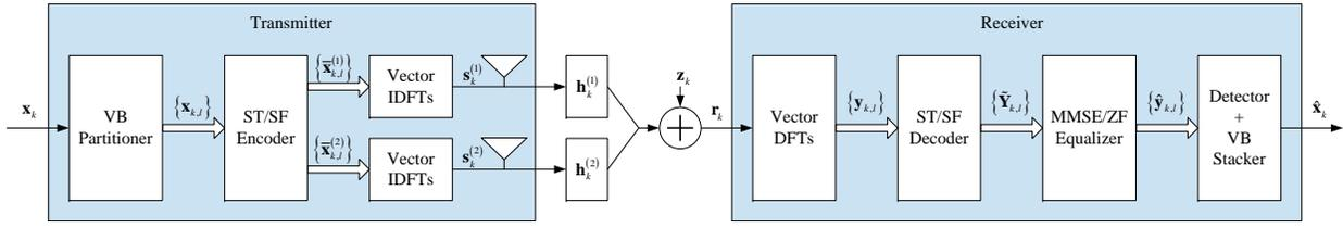
Fig. 1. Structure of the STBC and SFBC V-OFDM communication systems.
