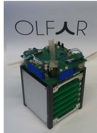
Figure 2: OLFAR antenna deployment mechanism prototype
