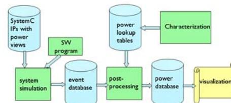
Figure 2. The SLEEP power estimation flow.
