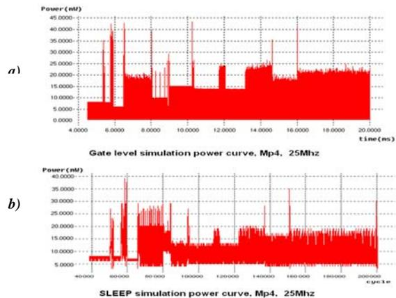
Figure 3. Simulation result of an MP4 decoder. We can observe a similar power profile between Diesel and the SLEEP simulation with a cache power model.
