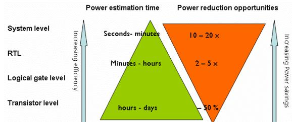
Figure 1. Power estimation in different design levels.
