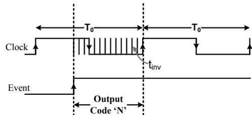
Figure 6 - ToF measurement technique for lower power consumption.
