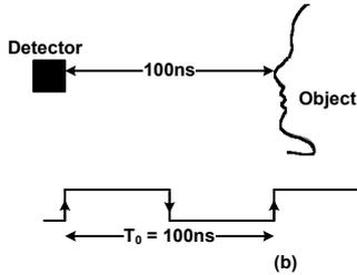
Figure 7 – The concept of Reconnaissance: (a) Lowest clock frequency when object is 30m (~200 ns) apart, (b) clock frequency increased when an object at closer distance is detected leading to lower power consumption.
