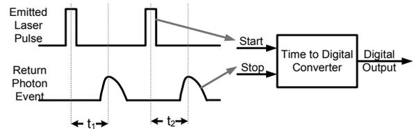
Figure 4 - Basic concept of TDC in 3D imaging.
