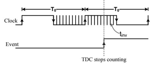
Figure 5 - Principle of a coarse-fine TDC [7].
