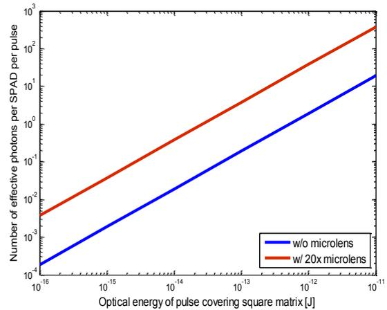
Figure 2 – Effective photons per SPAD per pulse vs. energy incident on a square matrix of detector.
