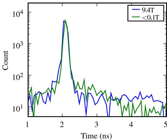
Figure 3: **GAPD jitter dependence on environment** — shown are jitter measurements of a circular, planar, 12 $\mu\text{m}$  GAPD under different magnetic fields. Delay measurements (x-axis) have been normalized so the peaks overlap.
