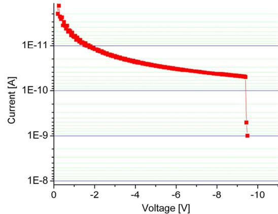
Figure 4. I-V Characteristic of the SPAD.
