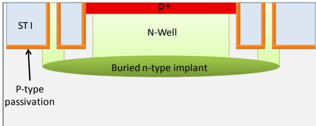
Figure 1. Cross-Section of the circular STI-bound SPAD (not to scale). The STI-interface is passivated using multiple p-type implants, thus reducing the probability of minority carriers entering the multiplication region and triggering dark counts.
