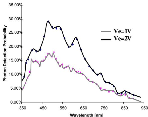
Figure 8. Photon detection probability for two different excess bias voltages.
