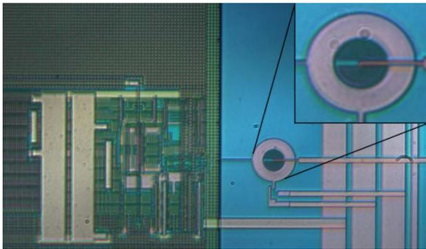
Figure 2. Photomicrograph of the SPAD and the integrated test electronics implemented in 130nm CMOS technology.
