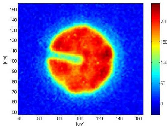
Figure 7. Measurement of the photoemission intensity (arbitrary scale) across the SPAD during avalanche breakdown. Uniform emission indicates equal probability of breakdown on the active area.
