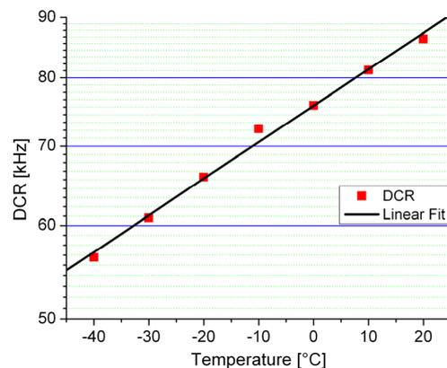
Figure 5. Dark count rate of the SPAD in function of temperature at 1V of excess bias voltage. The slope of the curve indicates that tunneling is the dominant noise source.
