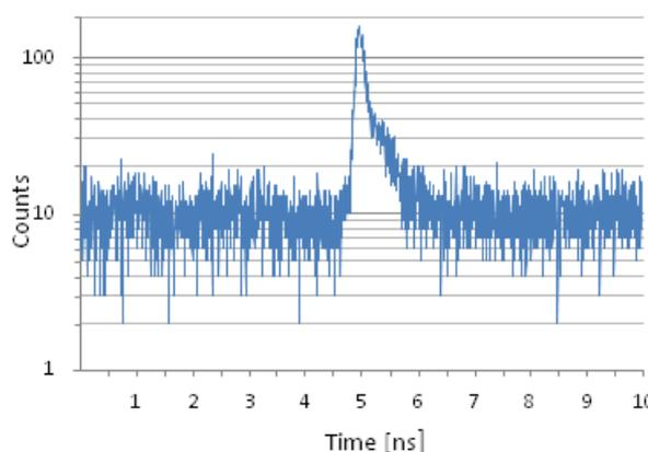
Figure 9. Time response of the SPAD when illuminated by a picosecond light source at 637nm wavelength and 1V of excess bias voltage.
