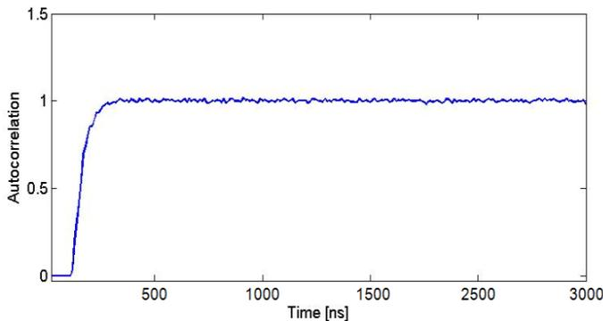
Figure 10. Autocorrelation probability of the SPAD. No afterpulsing contribution could be measured.
