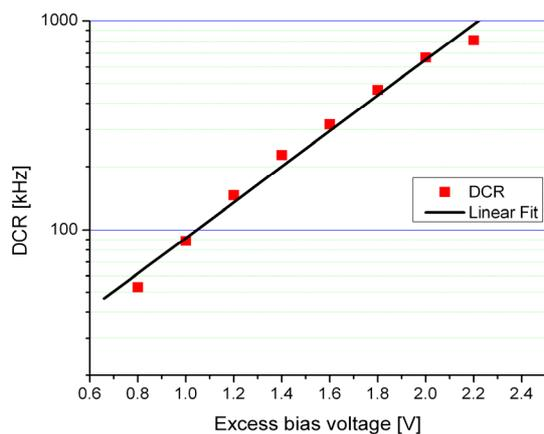
Figure 6. Dark Count Rate at room temperature as a function of the excess bias voltage.
