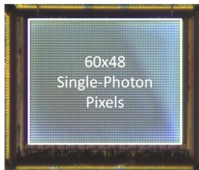
Figure 5. Photomicrograph of the SPSP image sensor. The circuit, fabricated in 0.35 $\mu$ m CMOS technology, has a surface of 6.5x5.5mm<sup>2</sup>. The pixel pitch is 85 $\mu$ m.
