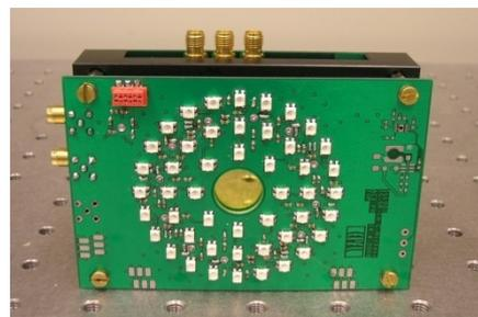
Figure 6. 3D camera prototype based on SPSP.
