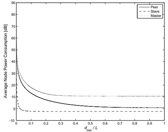
Fig. 4. Power requirements: average node power consumption as a function of  $d_{\min}/L$ .
