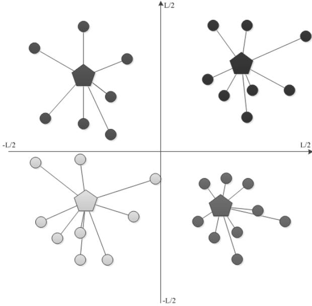
Fig. 2. Clustering example. The area over which the sensor network is spread was divided into four equal subareas, each one corresponding to a different cluster. The master nodes are represented by pentagon shapes, whereas the slaves are represented by circles.
