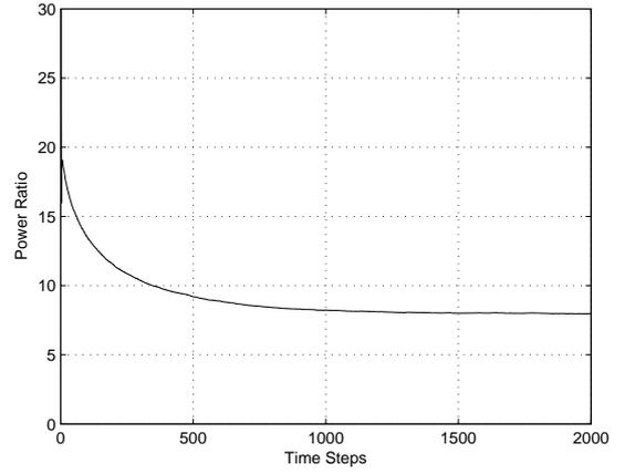
Fig. 7. Power Ratio: transmission power needed for a full-mesh topology divided by the transmission power necessary when applying the dynamic clustering scheme.
