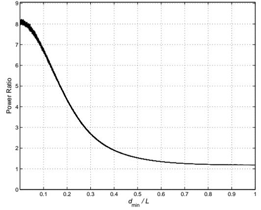
Fig. 3. Power-efficiency of clustering: the ratio between the necessary power for a full-mesh network and the necessary power for a clustered network as a function of  $d_{\min}/L$ .
