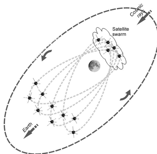
Fig. 1. Satellite swarm orbiting around the Moon. Eccentric orbiting causes the satellite cloud to vary its distribution with position.
