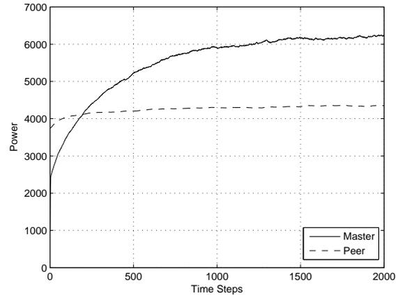
Fig. 10. Power Requirements: maximum transmission power for master nodes (clustering approach) and peer nodes (full-mesh topology).
