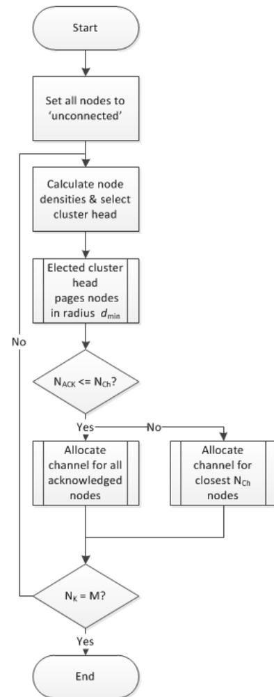
Fig. 5. Initial cluster formation. ( $N_{\text{ACK}}$  is the number of acknowledgment messages that an elected cluster head receives after paging,  $N_{\text{K}}$  is the number of formed clusters, and  $M$  is the desired number of clusters)
