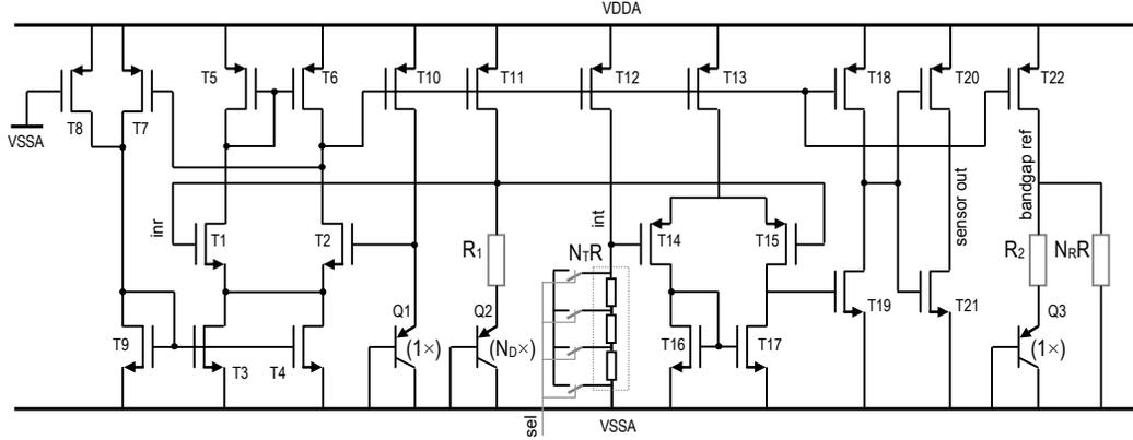
Figure 1: Temperature sensor – schematic view
