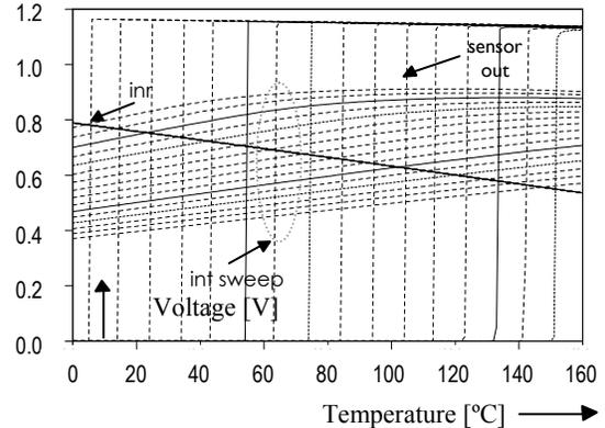
Figure 3: Sixteen selection levels in the temperature sensor
