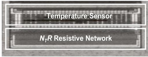
Figure 5: Chip micrograph
