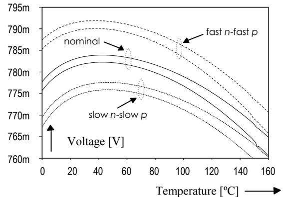
Figure 4: Bandgap reference voltage; nominal, fast-fast and slow-slow process corners
