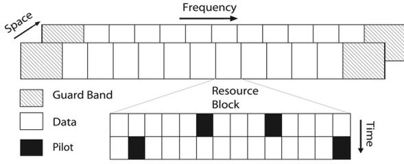
Fig. 1. Data structure of an OFDM block for a MIMO-OFDM/A downlink.
