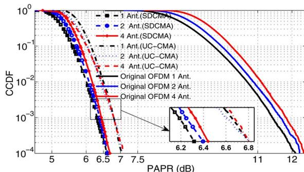
Fig. 5. PAPR reduction performance in MIMO-OFDM for both SDCMA and UC-CMA with 50 iterations and  $\mu' = 0.05$ .
