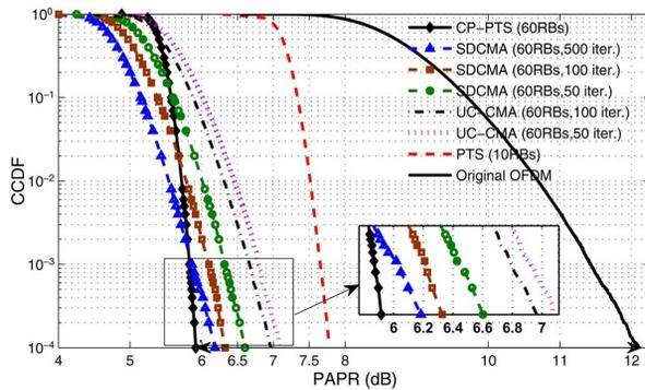
Fig. 3. Performance comparison for the proposed CMA PAPR reduction algorithm for various number of iterations and  $\mu' = 0.05$ , CP-PTS with 5 iterations, and conventional PTS with phase alphabet  $\{\pm 1\}$  and  $M = 10$ .
