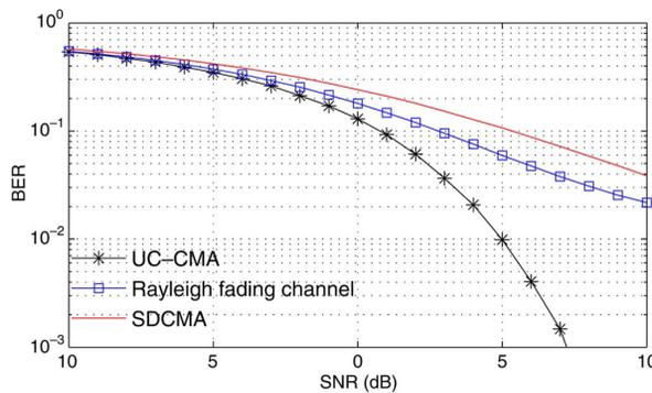
Fig. 4. BER performance of the proposed algorithms in comparison with AWGN and Rayleigh fading channels for single antenna QPSK-OFDM system of size  $N = 1024$  and  $M = 60$ .
