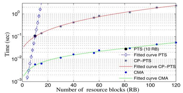
Fig. 6. Complexity comparison between CMA, CP-PTS and PTS using Matlab runtime evaluation.
