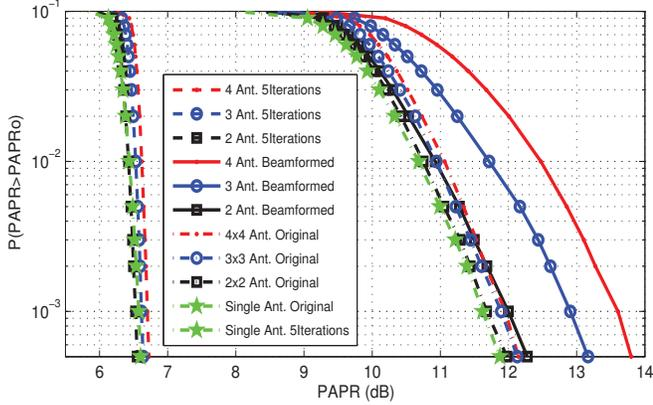
**Fig. 2:** CCDF curves of PAPR for 64QAM OFDM block with  $N = 1024$  and  $M = 60$ . The curves are plotted for different number of antennas and  $T = 2$ . Corresponding PAPR reduced CCDFs are derived with 5 iterations.
