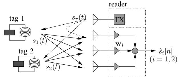
Fig. 1. Blind Source Separation scenario. The reader receives multiple overlapping tag signals, plus a copy of its own transmitted signal. A beamformer is used to recover each of the tags.
