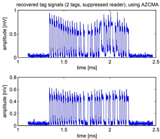
Fig. 8. Recovered tag signals (dataset with 2 tags and suppressed reader signal); beamformers computed using AZCMA
