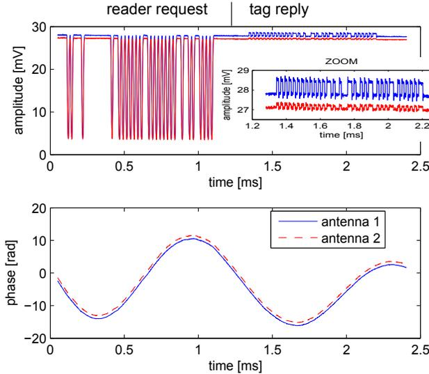
Fig. 4. Baseband amplitude and phase of a measured RFID reader and tag reply signal (2 antennas). Superimposed on the tag signal is the strong unmodulated reader carrier signal that provides power to the tags. Oscillator drift causes significant phase fluctuations.
