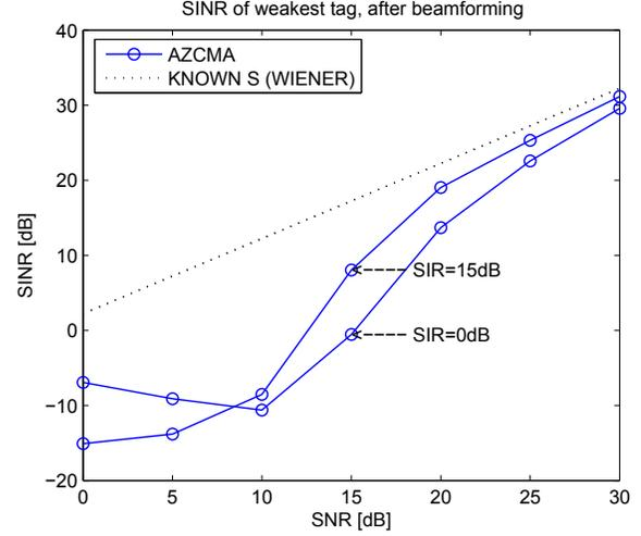
Fig. 6. SINR at the output of the beamformer vs. input SNR
