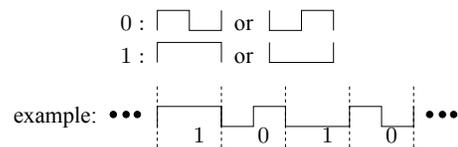
Fig. 2. FM0 symbol encoding [3]
