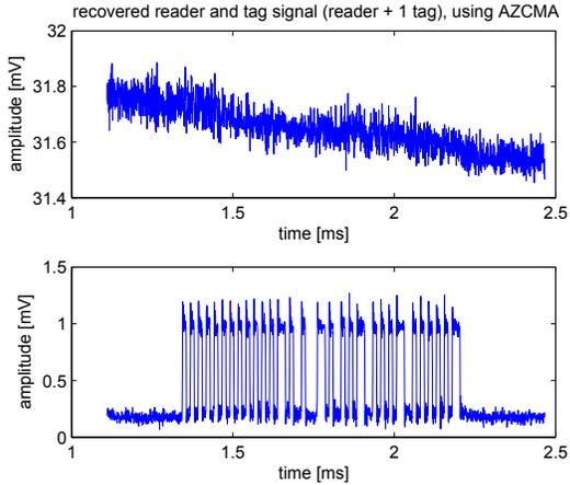
Fig. 7. Recovered reader and tag signal for the dataset in figure 4 (reader + 1 tag); beamformer computed using AZCMA
