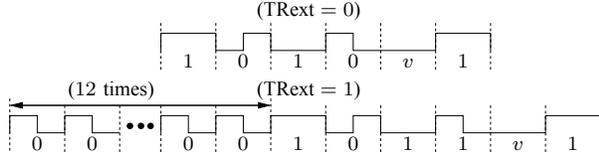
Fig. 3. FM0 preambles (two choices defined by parameter TRext) [3]
