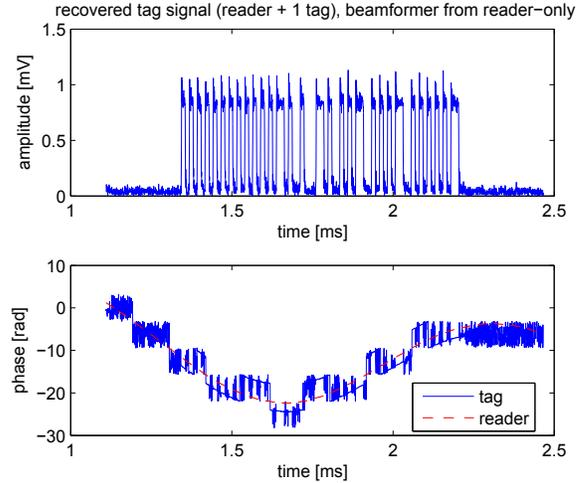
Fig. 5. Amplitude and phase of recovered tag signal for the dataset in figure 4 (reader + 1 tag); the beamformer is computed from the interval in which only the reader signal is present. The recovered phase somewhat follows that of the reader, but can be considered as random.
