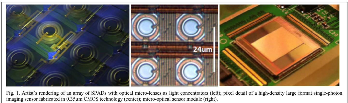
Fig. 1. Artist's rendering of an array of SPADs with optical micro-lenses as light concentrators (left); pixel detail of a high-density large format single-photon imaging sensor fabricated in 0.35µm CMOS technology (center); micro-optical sensor module (right).
