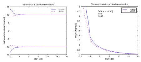
d=2 sources, M=6 antennas, N=40 samples,  $20^{\circ}$  separation.
