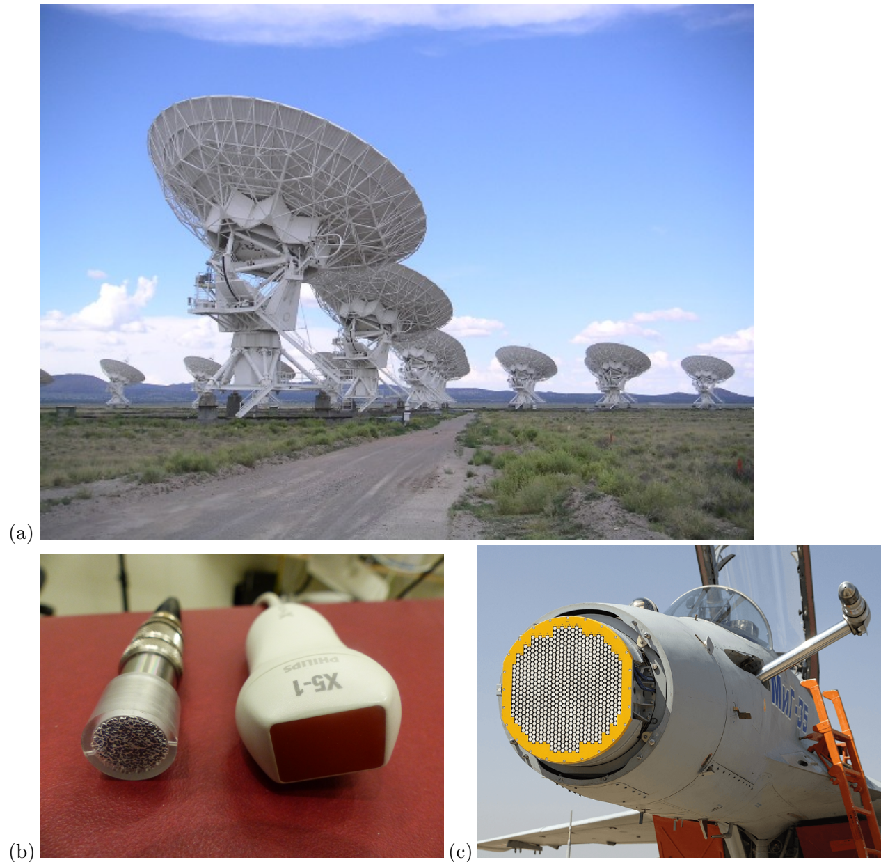
Figure 1.1. (a) Example of a radio telescope: The Very Large Array, New Mexico; (b) a single element ultrasound transducer next to a 3D ultrasound array; (c) MiG-35 phased array radar.
