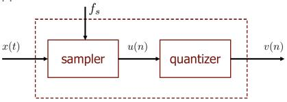
Basic task: convert a continuous range of input amplitudes to a discrete set of digital code words.
