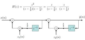
Let us consider a second-order filter H(z), which is a cascade of two first-order filter sections  $H_1(z)$  and  $H_2(z)$ .
