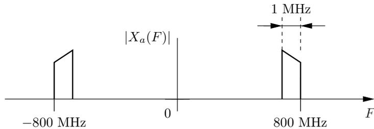
Think e.g. of a GSM signal at a carrier frequency slightly below 800 MHz.
