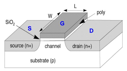
Position of switch depends on gate to source voltage
