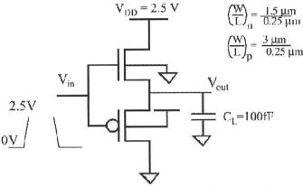
**a.** Write the equations for  $V_{OH}$  and  $V_{OL}$  taking into account the body effect in both transistors. First write it using symbols, than fill in numbers. You don't need to solve the equations.
