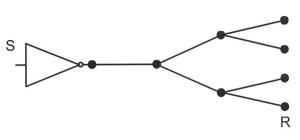
**a.** When the total capacitance of all segments together amounts to 1pF (which is not the correct answer to the next question), calculate the average current that the driver (the inverter) should deliver for a 50% delay of 1ns. For this question, please disregard the resistance of the wires. Assume  $V_{DD} = 2.5V$ .
