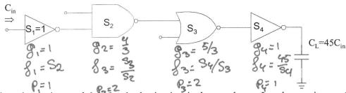
a. Calculate the optimum delay for the logic circuit shown above. Load capacitance  $C_L$  is 45 times the gate capacitance of the first inverter *Cin*. Determine the sizes S<sub>2</sub>-S<sub>4</sub> and the minimum delay expressed in term of  $t_{\nu 0}$  (intrinsic delay). Assume  $\gamma = 1$ .
