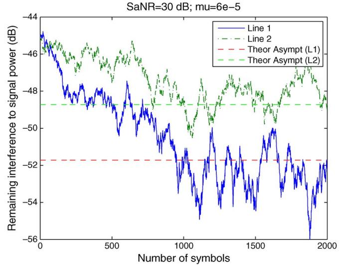
Fig. 5. Comparison between predicted (horizontal dashed lines) and simulated asymptotic performance.
