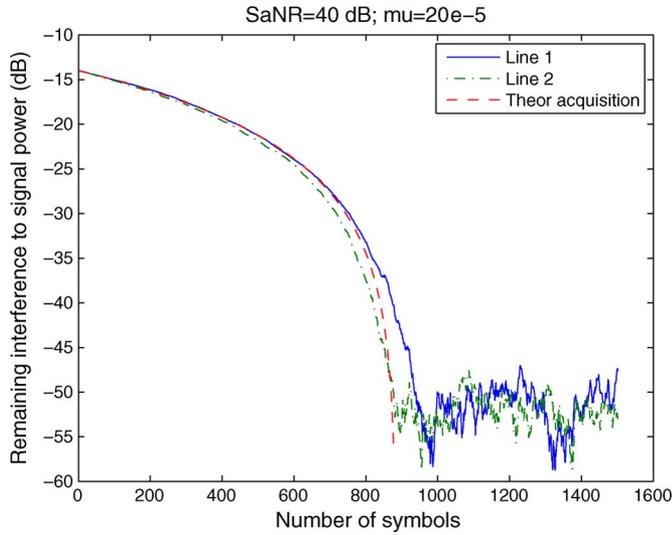
Fig. 3. Comparison between predicted (dash line) and simulated acquisition speed (SaNR = 40 dB, initial crosstalk at 14 dB).
