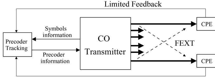
Fig. 1. Principle of the structure for the iterative precoder algorithm.
