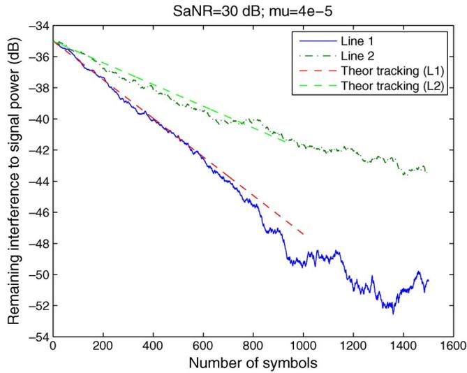
Fig. 4. Comparison between predicted (dashed line) and simulated tracking speed.
