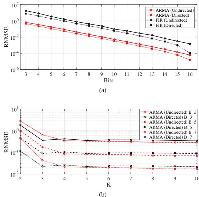
Fig. 8. Average RNMSE of linear prediction on the Molene temperature data set. (a) Average RNMSE of the approximated signal as a function of the number of bits ( $B$ ) for filter order  $K = 3$ . (b) Average RNMSE of the estimated signal for different order ARMA filters evaluated for  $B = 3, 5, 7$ .
