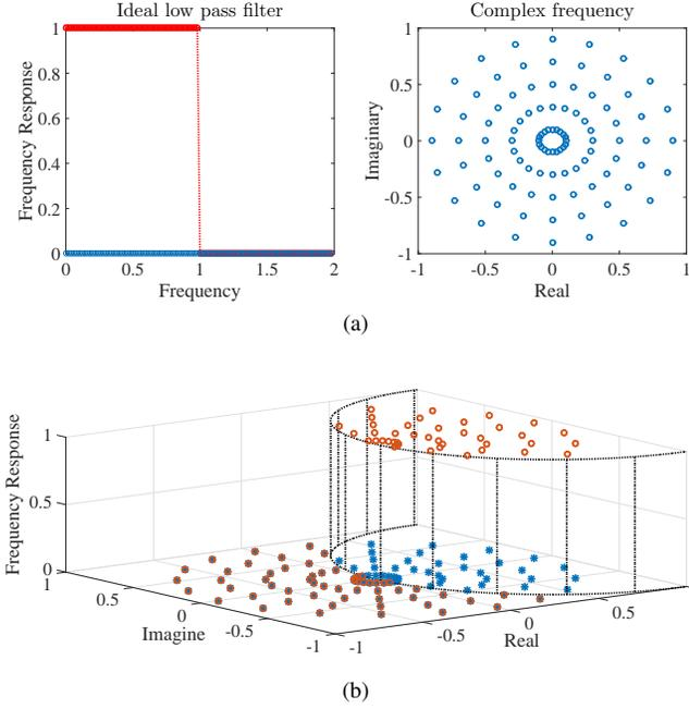
Fig. 2. (a) (left) Ideal low pass filter response of universal design for undirected graph ( $N = 100$ ). (a) (right) Universal gridding for directed graph associated with the normalized adjacency matrix  $\mathbf{A}_n$  ( $N = 100$ ). (b) Ideal low pass filter response of universal design for directed graph with  $N = 100$ . The complex frequencies lying inside the circle with radius 1 centered at  $(1, 0)$  are “small” frequencies.
