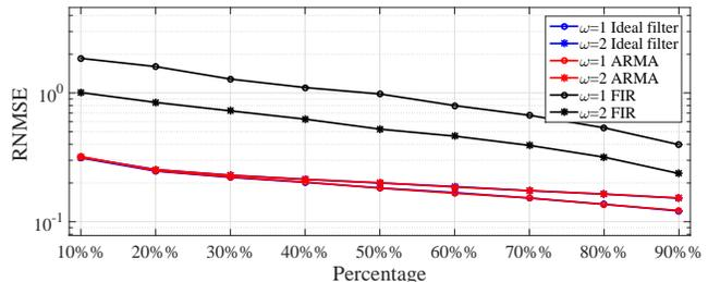
Fig. 6. RNMSE of the ARMA graph filter for interpolation of the Molene data set, where  $\omega = 1, 2$ . As two comparisons, ideal graph filter and FIR filter with order  $K = 20$  are shown with the same values of  $\omega$ .
