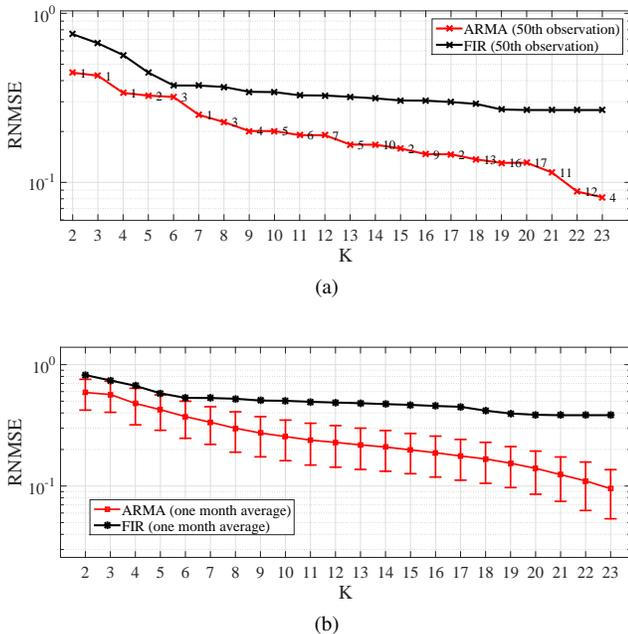
Fig. 7. RNMSE between the data spectrum and the filter frequency response as a function of filter order  $K$ . (a) Illustration of the RNMSE of the ARMA graph filter and the same order FIR filter for the 50th observation. The order  $Q$  is shown in the plot and  $P + Q = K$ . (b) Average RNMSE over all 744 temperature realizations (one month) for different filter orders. For the ARMA filter, each error bar shows the standard deviation of the approximation error for order  $K$ .
