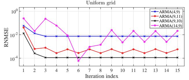
Fig. 4. RNMSE of the iterative approach on the universal design with  $N = 100$  points. Performance evaluation for different ARMA filters which are a few particular cases illustrating monotonic convergence, non-monotonic convergence, and no convergence.
