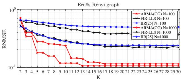
Fig. 5. RNMSE of the ARMA graph filter implementation on an Erdős Rényi graph with  $N = 100$  and  $N = 1000$ . Performance evaluation for the trade-off between computational cost and approximation accuracy. For CG, the complexity of the ARMA implementation is limited by  $PT + Q \leq K$ .
