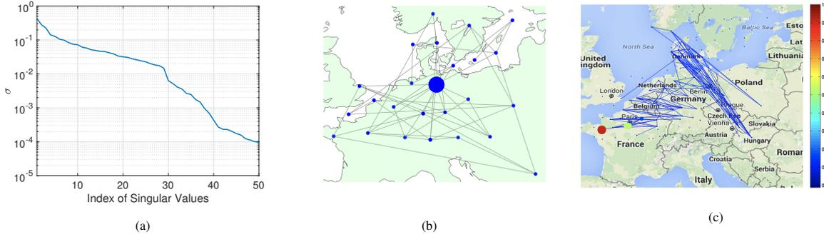
**Fig. 2:** (a) First 50 singular values ( $\sigma$ ) of  $\frac{1}{m} \mathbf{Y}_m$  for  $m = 3 \times 10^4$  and  $s = 169$ . Here, the original dataset has been interpolated and filter to increase the length of the recordings. The first knee, i.e., the drop in singular values (SV), occurs at the 5th SV, the second drop happens around the 20th SV. (b) Learned graph from dataset using the proposed one-shot state graph estimator. (c) Learned graph in [34] using the ETEX dataset.
