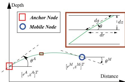
Fig. 1. Ray path between a mobile node and an anchor node.
