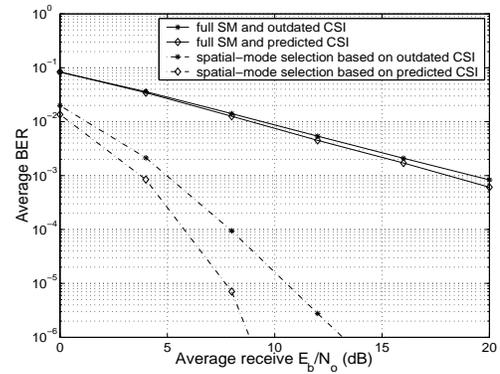
Figure 1: Illustration of the performance of spatial-mode selection based on channel mean feedback for a (4,4) MIMO setup, using the robust MMSE design, at spectral efficiency of 8 bits/s/Hz and normalized delay  $f_D T_{obs} = 0.1$
