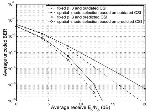
Figure 2: Illustration of the performance of spatial-mode selection based on channel mean feedback for a (4,4) MIMO set-up, using the robust MMSE design, at spectral efficiency of 12 bits/s/Hz and normalized delay  $fd.T_{obs} = 0.1$
