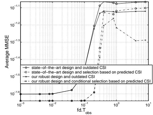
Figure 3: Average MMSE versus the normalized delay for a (4,4) MIMO set-up with 3 streams at spectral efficiency of 12 bits/s/Hz,  $E_b/N_o = 20$  dB and using a  $2^{nd}$ -order linear MMSE predictor
