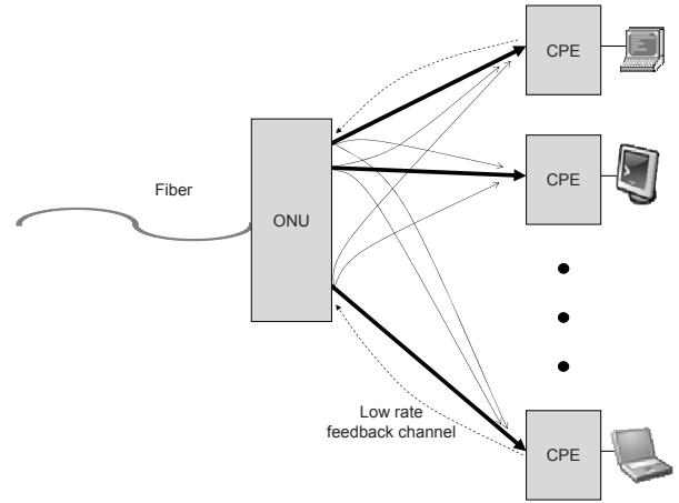
Fig. 1. Network topology with fiber to the point (FTTB/FTTC/FTTN) topology. Bold lines from ONU to CPE are the channels, thin lines are the far end crosstalk (FEXT) coupling channels.
