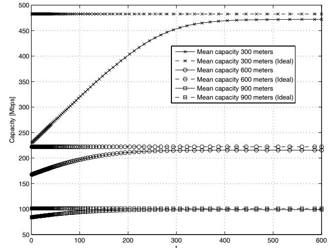
Fig. 5. Convergence of users' capacities at distances of 300, 600 and 900 meters in a mixed binder.
