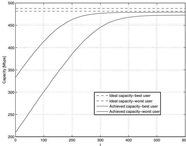
Fig. 4. Convergence of best and worst users' capacities at a distance of 300m.
