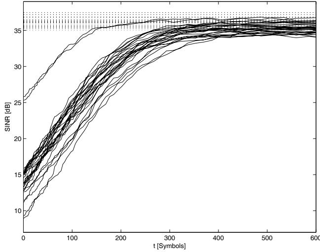
Fig. 2. SINR Convergence at a distance of 300m and a frequency of 27.4MHz (28 users).
