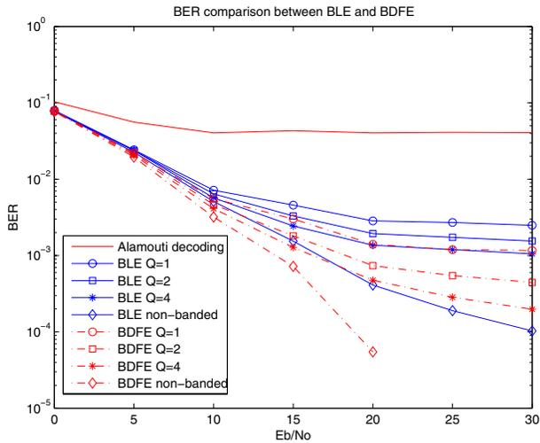
Fig. 3. BER comparison between BLE and BDFE
