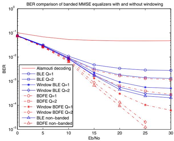
Fig. 4. BER comparison of banded MMSE equalizers with and without windowing
