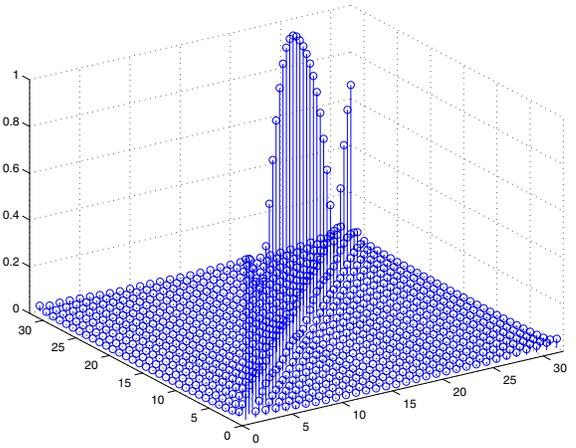
Fig. 2. An example of a frequency-domain channel matrix ( $N = 32$ )
