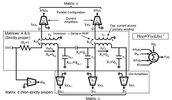
Fig. 1. Generic orthonormal transformer-C state space filter
