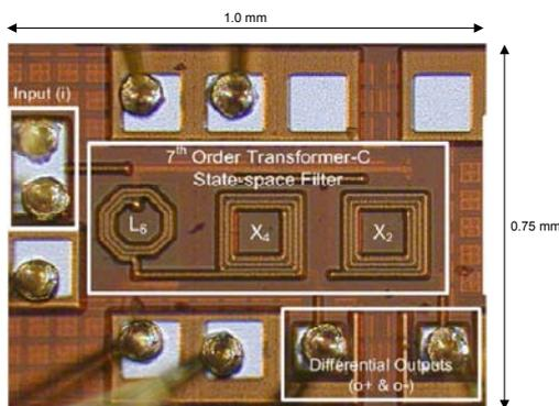
Fig. 8. Chip microphotograph of the 7<sup>th</sup> order orthonormal *transformer-C* state-space filter in  $0.13 \mu\text{m}$  CMOS technology; active area is  $0.15 \text{ mm}^2$ ; physical dimensions are  $(0.625 \times 0.25) \text{ mm}$
