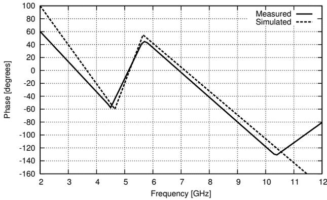
Fig. 6. Phase response of the band-reject filter
