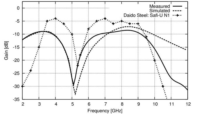
Fig. 5. Magnitude response of the 7<sup>th</sup> order orthonormal transformer-C state space band-reject filter (without de-embedding)
