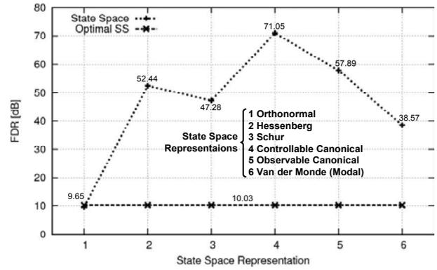
Fig. 3. FDR comparison for different state-space descriptions of a 7<sup>th</sup> Daubechies' scaling function
