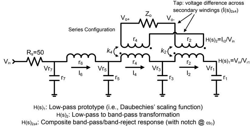
Fig. 4. 7<sup>th</sup> order orthonormal transformer-C state space band-reject filter
