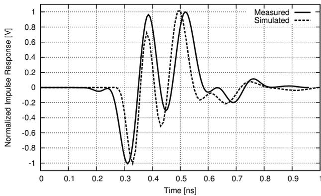
Fig. 7. Impulse response of the band-reject filter
