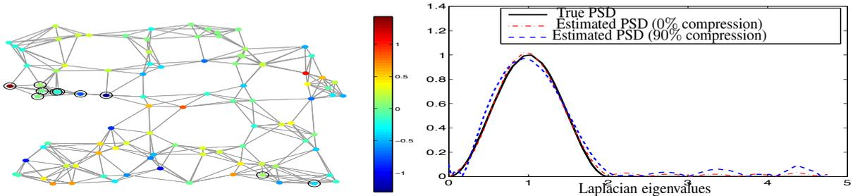
**Fig. 2:** Graph vertex domain subsampling. Left: Random graph with  $N = 100$  nodes. Sampled  $K = 10$  nodes are depicted with a black circle. Right: Graph power spectrum, where the true power spectrum is modeled with  $Q = 12$ .
