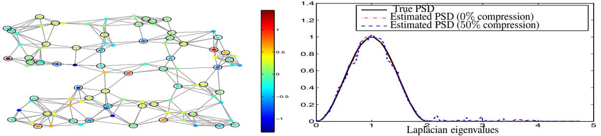
**Fig. 1:** Graph spectral domain subsampling. Left: Random graph with  $N = 100$  nodes. Sampled  $K = 50$  nodes are depicted with a black circle. Right: True and estimated graph power spectrum.
