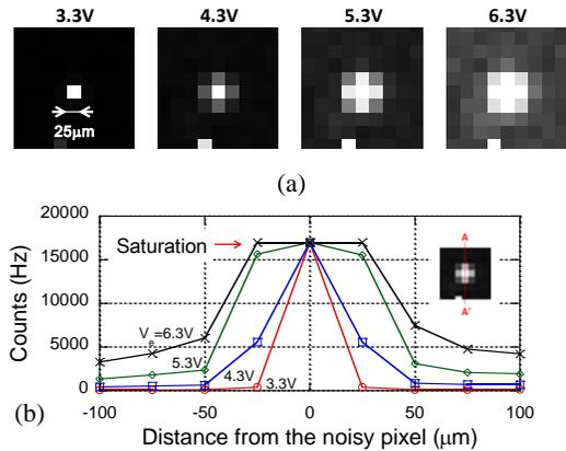
Fig. 3. (a) Close-up images of a hot pixel taken in the dark at various  $V_e$  from 3.3V to 6.3V. The images clearly show that the optical crosstalk is dominant over electrical crosstalk. (b) DCR distribution around a hot pixel. The photon emission from a hot pixel raises the DCR in neighboring pixels, which are located  $25\mu\text{m}$  to  $75\mu\text{m}$  away.
