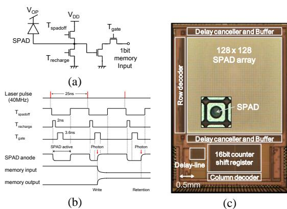
Fig. 1. (a) Schematic diagram. (b) Timing diagram. (c) Chip photomicrograph of the sensor. Time gating is achieved through transistors  $T_{\text{spadoff}}$ ,  $T_{\text{recharge}}$  and  $T_{\text{gate}}$ . The column decoder is used to serialize the data coming from the array onto two serial channels via the 16-bit shift register. The chip was fabricated in a  $0.35\mu\text{m}$  HV CMOS technology. The pixel pitch and a total area are  $25\mu\text{m}$  and  $20.5\text{mm}^2$ , respectively.
