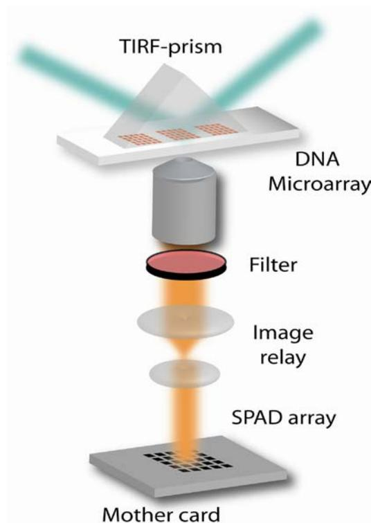
Fig. 1. Experimental setup of the TIRF-SPAD imager setup. (see text for details).
