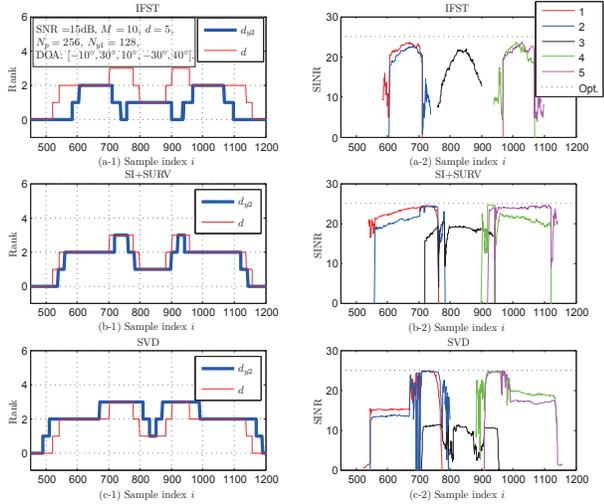
Fig. 4.2. The rank estimates and SINR of the beamformers for packets in one run.
