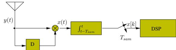
Figure 1: Autocorrelation receiver
