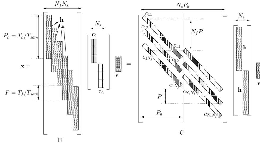
Figure 3: The data model for the single user, single delay case (time offset not shown)
