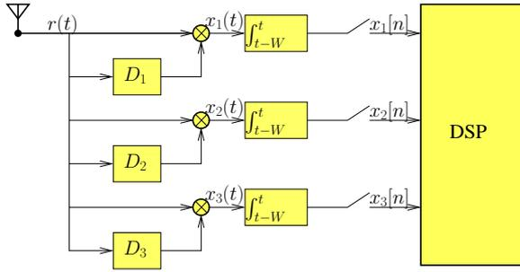
Figure 4: Receiver structure with multiple correlators
