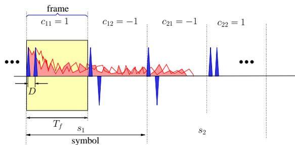
Figure 2: Pulse sequence structure
