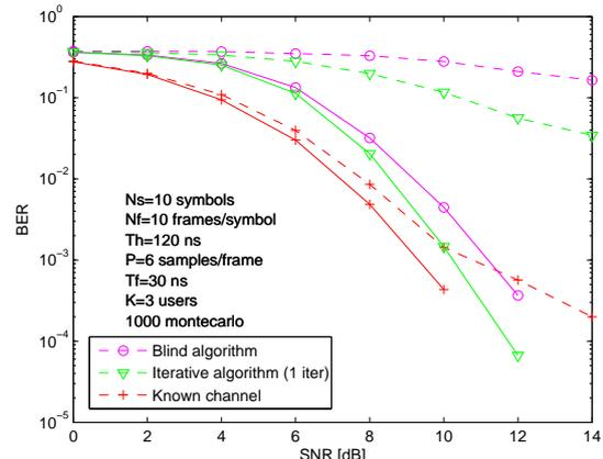
Figure 5: BER vs. SNR performance comparison between single delay and multi-delay schemes for CM2. Solid: multiple delays ( $M = 4$ ), dashed: single delay ( $M = 1$ ).
