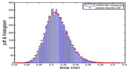
Fig. 4. The *pdf* and histogram comparison of AOI22
