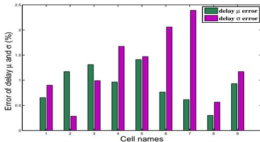
Fig. 5. First-order voltage sensitivity calculation method for delay distribution computation of standard cells. The numbers of 1 to 9 stand for INV, NAND2, NOR2, BUF, AND2, XOR2, AOI211, NAND4 and MUX2 respectively [16].
