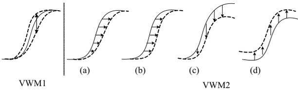
Fig. 1. The variational waveform models VWM1 and VWM2
