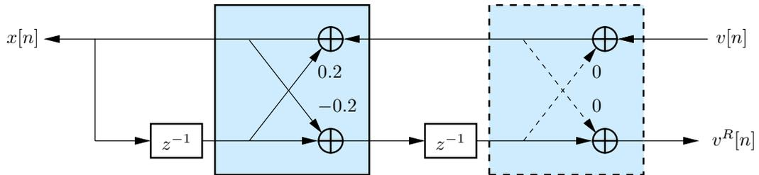
This is obtained by “reversing” the signal flow of  $v[n]$  to  $x[n]$  in the previous figure while maintaining the same relations between variables.
