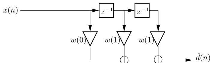
The filter has three tap coefficients, but  $w(1)$  and  $w(2)$  are equal. The goal is to find the two filter coefficients  $w(0)$  and  $w(1)$  that minimize the mean square error (MSE)
