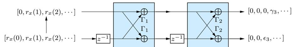
Starting from this, derive a lattice filter implementation that, given the reflection coefficients and  $r_x(0)$ , generates the rest of autocorrelation sequence at one of its outputs. (Specify also the input of the filter.)
