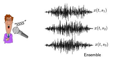
Sample function: one realization of the waveform x(t, s)
