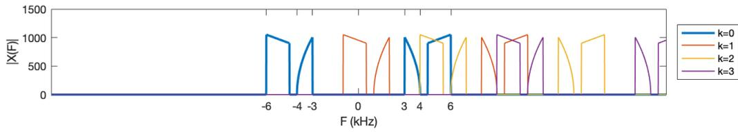
**Figure 1.** A sketch of the spectrum of the sampled signal can be helpful to write the equations: The spectrum of the analog signal is shown in blue. The periodic copies due to sampling are shown in red, yellow and purple. The highest frequency of the red copy must not be larger than 3kHz, while the lowest frequency of the yellow copy must not be smaller than 4kHz.
